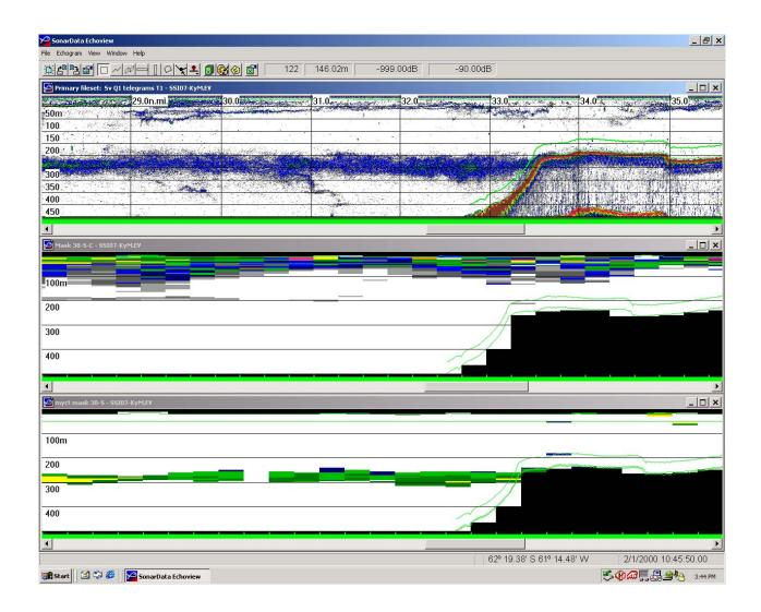
Figure 5. Example of echograms produced with Sonardata EchoView software. The top panel represents the original 38 kHz echogram, the second panel represents a filtered echogram containing krill only, and the third panel represents the same echogram containing myctophid fish only.
